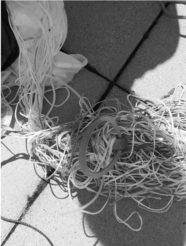
*Picture 4 shows the strong and firm entanglement of the handle with the suspension lines of the reserve parachute. The accident equipment arrived at the DHV for investigation in this condition.*
